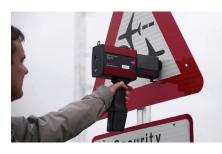
Mobile instrument A mobile device is typically used in large airports and when frequent retroreflective measurements are to be made. DELTA's LTL-M mobile retroreflectometers measure
